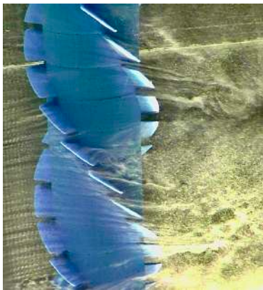
Figure 14: Detail of flow visualization with hydrogen bubbles for continuous and serrated strakes. Re = 9.4 \times 10^3 .
