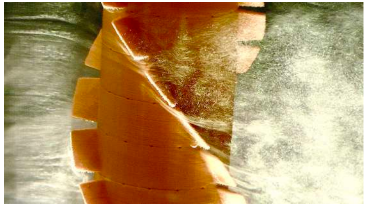
(a) S30 serrated 30-strake.
